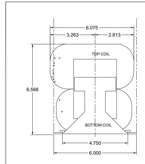
OPTION - FLIPPING COILS TO HAVE LEAD EXITS ON OPPOSITE SIDE OF TRANSFORMER TO MAINTAIN CHASSE WALL CLEARANCE - ADDITIONAL LENGTH WOULD BE ADDED TO LEADS TO ACCOMMODATE NEW ORIENTATION
